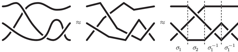
FIGURE 1. Normalization of a braid diagram and expression as a product of elementary diagrams \sigma_i et \sigma_i^{-1} .
